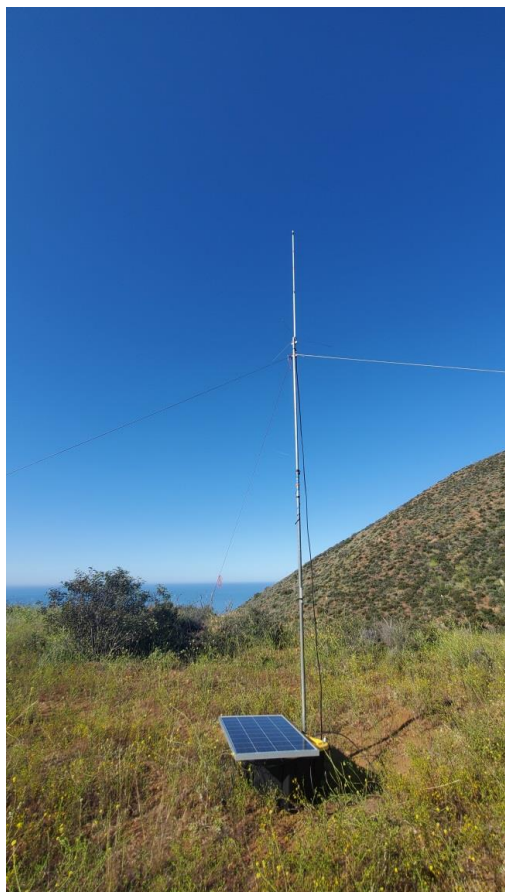
This shows the club's 20 foot push-up mast with a Tram 1480 high gain Omni directional antenna up on Overlook Fire road.
